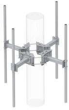
4-sector Monopole 24" Stand-off Mount kit, 10 in to 30 in OD, includes (4) 2-7/8" OD x 96" pipe
