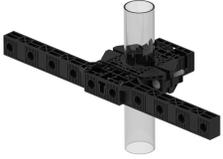
Polymer PIM-Guard® Antenna and RRU Cable Support Bracket - Extra Wide with 18 positions for stackable hangers (up to 2 per position)
