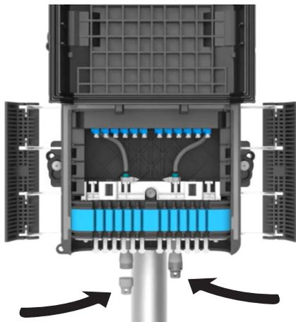
Gently remove the dust caps from the HFMOC connectors located at the bottom of the junction box. Ensure that the connectors remain clean and free from contaminants during the process. Carefully remove the dust caps from the HFMOC connectors on the FT-24CGAHBN series cable, taking care not to touch or contaminate the fiber ends.
