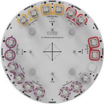
16-port small cell antenna, 4x 698-896, 4x 1695-2690 and 8x Beamforming 3300- 4000, 360° Horizontal Beamwidth, fixed tilt.
