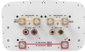
6-port Next Generation High Performance sector antenna, 2x 698-894 and 4x 1695-2360 MHz, 65° HPBW, 3x RETs and 2x SBTs.
