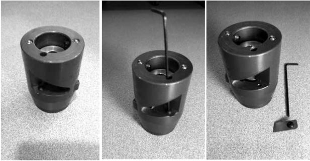
Remove the 6-32" button head screw holding the flat outer conductor blade in place. Insert the 5/64" hex key through the small hole in the top of the tool under the flaring tool. Debris should fall from the tool. If needed, pick, shake, or use compressed air to remove any adhering debris.
