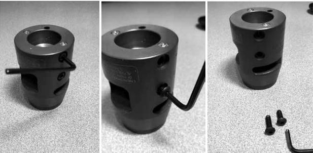
Remove the two 1/8" button head screws on the side of the tool with the supplied 1/8" hex key.
