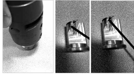
Once the assembly has been removed from the housing, most of the debris will fall from the tool. Using the supplied hex key, drag the hex key along the underside of the blade in the direction of the blade and any excess material will pull away from the blade. If needed, pick, shake, or use compressed air to remove any adhering debris from the blade or tool body. Reassemble blades in the reverse order shown. **CAUTION! Do not over-tighten screws.**
