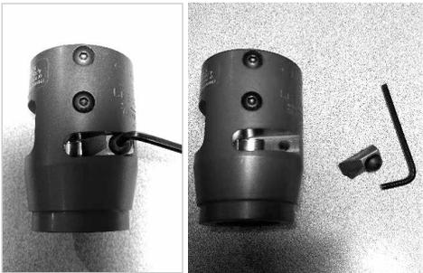
Remove the jacket stripping blade using the 1/8" hex key. Debris should fall from the tool. If needed, pick, shake, or use compressed air to remove any adhering debris.
