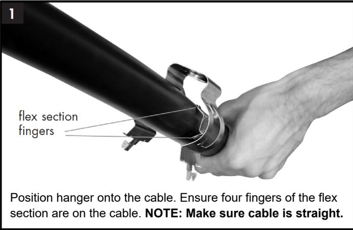
Position hanger onto the cable. Ensure four fingers of the flex section are on the cable. **NOTE: Make sure cable is straight.**
