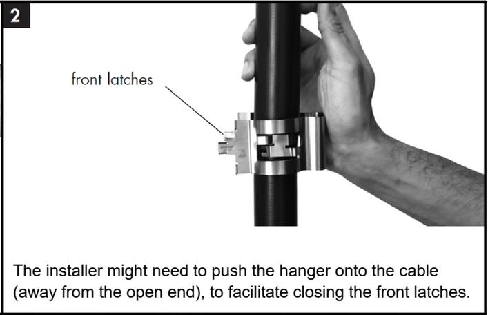
The installer might need to push the hanger onto the cable (away from the open end), to facilitate closing the front latches.
