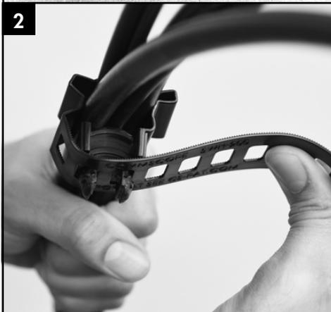
Stretch and wrap strap tightly around cable bundle expanding the corrugations until you get two strap holes to slide down onto the latches.
