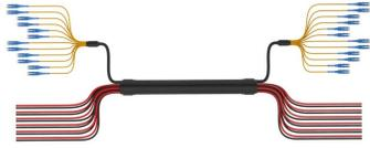
HELIAX® Hybrid Cable Assembly, 6 X 12, 12 X 4AWG 19-Strand Conductors, 24 SM Fiber, DLC-DLC, PVC jacket, Cu Foil Shield
