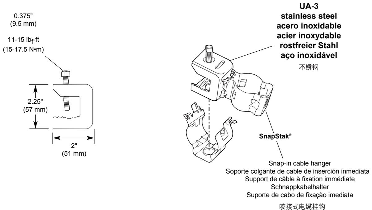
Type UA-3 adapters are designed for mounting 1/2" to 1-5/8" SnapStak® snap-in hangers to angle or round tower members. The adapters are also compatible with standard HELIAX® hangers by using insert UAAI (not included).
