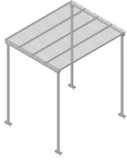
Ice Canopy, 8 ft x 8 ft, four 10 ft 6 in base shoe pipes
