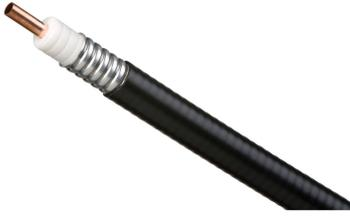
AL5-50, HELIAX® Low Loss Flexible Aluminum Coaxial Cable, corrugated aluminum, 7/8 in, black non-halogenated, fire retardant polyolefin jacket.
