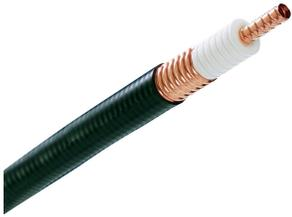
AVA7RK-50, HELIAX® Andrew Virtual Air™ Coaxial Cable, corrugated copper, 1-5/8 in, black non-halogenated, fire retardant polyolefin jacket Cca-s2, d2, a1 (CPR testing is conducted annually please reference the website for latest classification)
