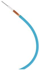
PTS1-50, HELIAX® Superflexible High Power, High Temperature 50 Ohm Plenum Rated Coaxial Cable, corrugated copper, 1/4 in, blue PVDF jacket
