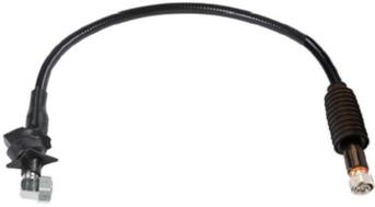
HELIAX® 1/2" Superflexible Fire retardant SureFlex® Jumper with interface types 7-16 DIN Male and 7-16 DIN Male Right Angle with HELIAX® SureGuard weatherproofing, 3m, with black non-halogenated fire retardant polyolefin jacket B2ca-S1a-d1-a1
