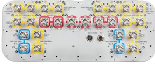
26-port sector antenna, 2x 694-862 (R1), 2x 880-960 (R2), 2x 694-960 (R3), 4x 1427-2690 (Y3/Y5), 4x 1695-1880 (B1-B2), 4x 2300-2690 (Y1&Y7) & 8x 1695-2690 (Y2/Y4/Y6/Y8) MHz, 65° HPBW, 8x RET.
