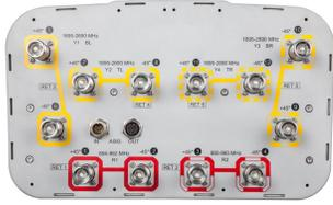
12-port multiband antenna, 2x 694–862, 2x 880–960 and 8x 1695–2690 MHz, 65° horizontal beamwidth, 6x Internal RET. Low band arrays are diplexed at the element level.
