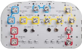
14-port sector antenna, 2x 694-862 (R1), 2x 880-960 (R2), 2x 1427-2690 (Y2), 4x 1695-2180 (B1-B2), 4x 2490-2690 (Y1 & Y3) MHz, 65° HPBW, 6x RET. Y1 & Y3 share a common RET
