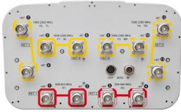
12-port sector antenna, 2x 698-803, 2x 824-894 and 8x 1695-2360 MHz, 65° HPBW, 4x RETs and low bands have diplexers.
