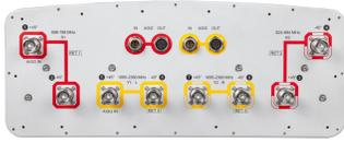
8-port sector antenna, 2x 698–798, 2x 824–894 and 4x 1695–2360 MHz, 45° HPBW, low bands each have a RET and the high bands share a RET. Two internal SBTs.
