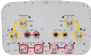
8-port sector antenna, 2x 698–803, 2x 824–894 and 4x 1695–2360 MHz, 65° HPBW, 3x RETs, low bands have diplexers. Internal SBT's on first LB(Port 1) and first HB(Port 5).
