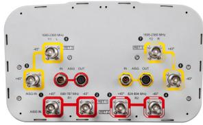
8-port sector antenna, 2x 698–787, 2x 824–894 and 4x 1695–2360 MHz, 65° HPBW, 3x RET and low bands have diplexers. Internal SBT's on first LB(Port 1) and first HB(Port 5).
