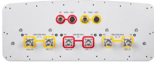
6-port sector antenna, 2x 698–896 and 4x 1695–2360 MHz, 45° HPBW, 2x RETs and 2x SBTs. Both high bands share the same electrical tilt.
