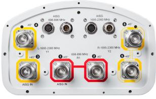
6-port sector antenna, 2x 698–896 and 4x 1695–2360 MHz, 65° HPBW, 2x RET. Both high bands share the same electrical tilt.
