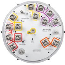
14-port quasi-omni antenna, 4x 698–896, 4x 1695–2690, 4x 3400–3800 and 2x 5150–5925 MHz, 360° horizontal beamwidth. Fixed and manual tilt.
