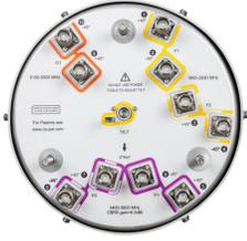
10-port small cell antenna, 4x 1695–2690, 4x 3400–3800 and 2x 5150–5925 MHz. 360° Horizontal Beamwidth, MANUAL ELECTRICAL TILT
