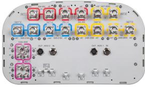
22-port sector antenna, 2x 694-862 (R1), 2x 880-960 (R2), 2x 1427-2690 (Y2), 4x 1695-2180 (B1-B2), 4x 2490-2690 (Y1 & Y3) MHz, 65° 8x 3300-3800 (P1) HPBW, 7X RET. Y1 & Y3 share common RET.
