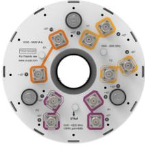
10-port small cell antenna, 4x 1695–2690, 4x 3300–4200 and 2x 5150–5925 MHz. 360° Horizontal Beamwidth, fix tilt
