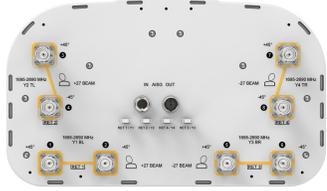
8-port multibeam antenna, 8x 1695–2690 MHz, 4x 33° HPBW, 4x RET, has tilt scales
