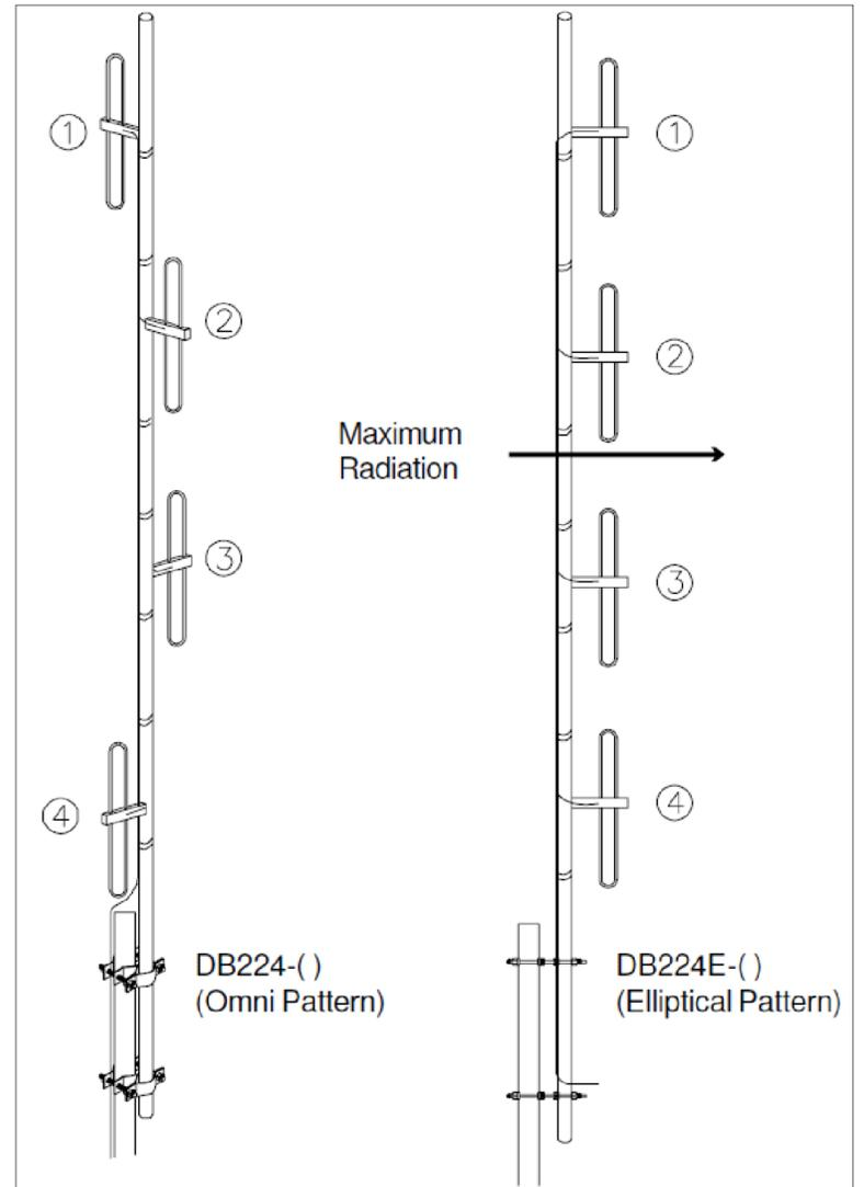
Figure 1. Dipole Alignment
