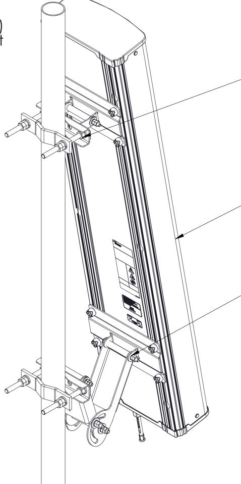
Bottom (standard pipe mount) assembly is attached to the top antenna bracket. 底部(标准管柱安装)组件安装到天线上部的安装托架。
