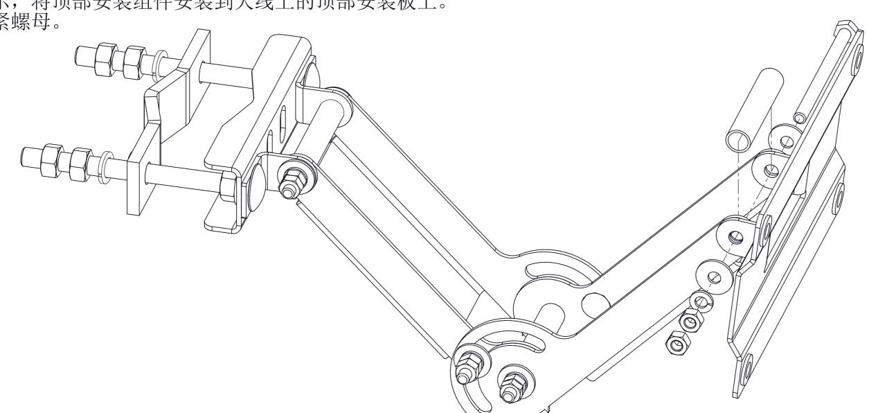
NOTE: To obtain a negative angle (e.g.  $-2^{\circ}$ ), attach the top (downtilt) assembly to the bottom antenna bracket.
