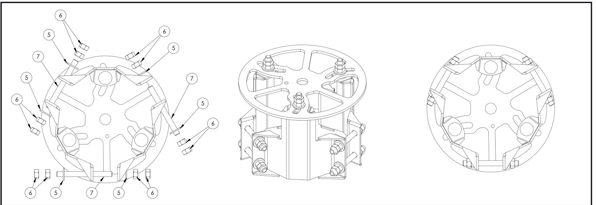
*INSTALL PIPE MOUNT BRACKET HARDWARE*
