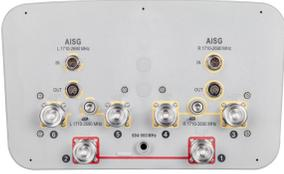
6-port sector antenna, 2x 694–960 and 4x 1710–2690 MHz, 65° HPBW, fixed electrical tilt (12°) low band, 2x RET on both high band arrays with a separate pair of AISG Input and Output ports per array.
