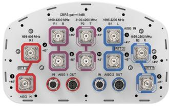
10-port sector antenna, 2x 698–896, 4x 1695–2200 and 4x 3100–4200 MHz, 65° HPBW, 2x RETs and 2x SBTs. Both high bands share the same electrical tilt.
