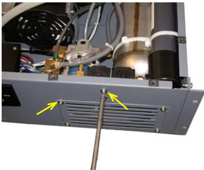
Step 3 Remove screws to detach filter assembly and front filter access panel from chassis.
