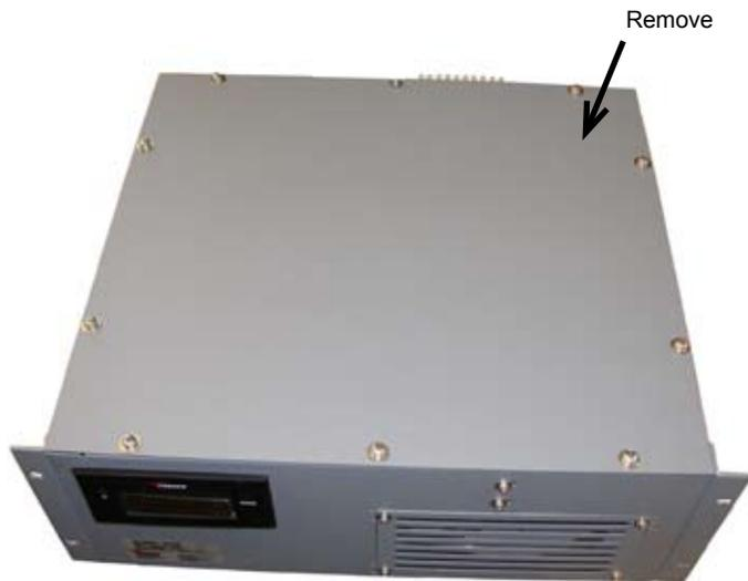
Step 1 Remove top cover of unit by removing (10) screws on top.
