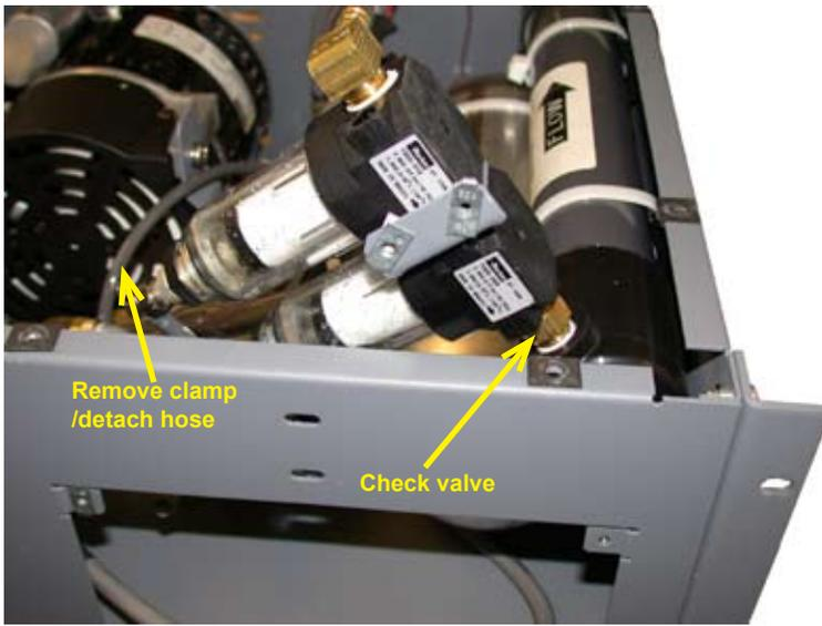
Step 4 Remove clamp from hose and detach hose from barb fitting on the bottom of filter assembly.
