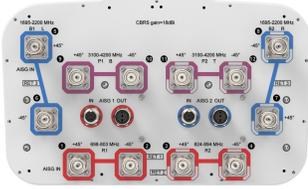
12-port sector antenna, 2x 698-803, 2x 824-894, 4x 1695-2200 and 4x 3550-3700 MHz, 65° HPBW, 3x RETs and 2x SBTs.
