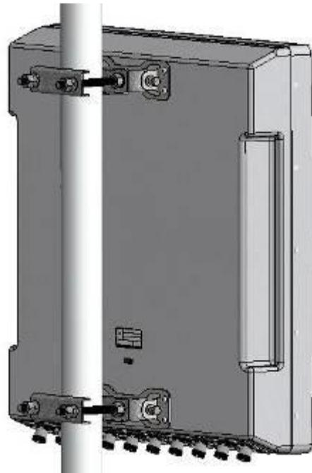
**Figure 1. Correctly Assembled Mounting Brackets**
