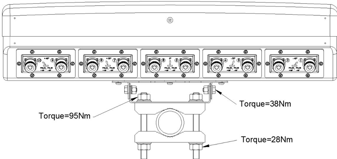
**Figure 2. Fixed Downtilt Mounting Bracket Assembled to Antenna & pole**
