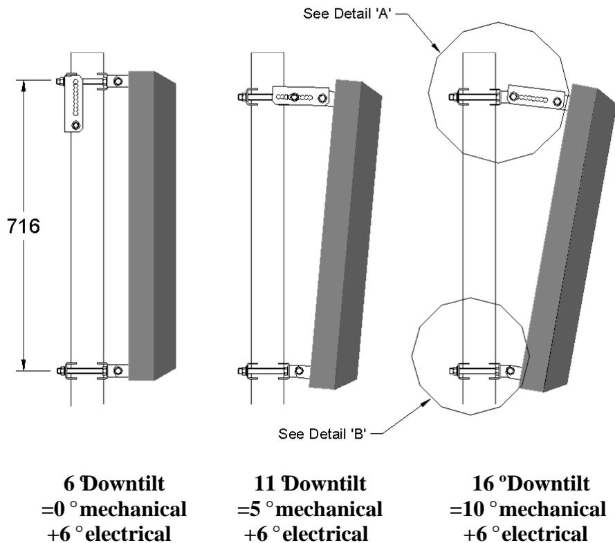
**Figure 5.** Setting mechanical down-tilt
