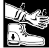
Wear shoes with rubber soles and heels. Wear protective clothing including a long-sleeved shirt and rubber gloves.
