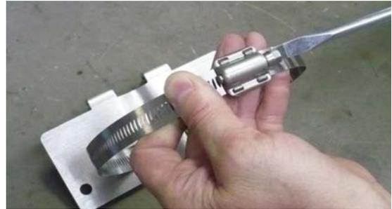
**Step 5** - Tighten the screw along the band up to the required torque (recommended 7.5 to 10Nm max) by means of a screwdriver
