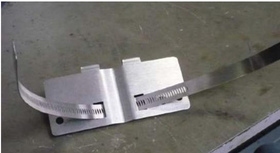
**Step 3** - Insert clamp into bracket
