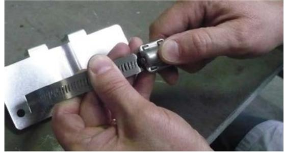
**Step 4** - Insert the free terminal of the clamp into lock
