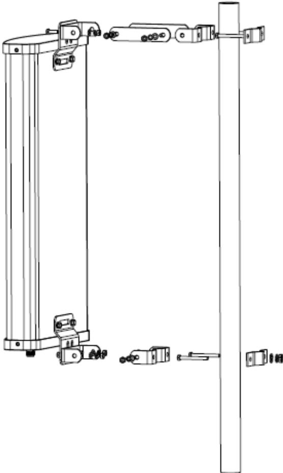
The antenna can be mounted to mounting hardware with a diameter of  $\Phi$  25 mm to 60 mm with supplied clamps.
