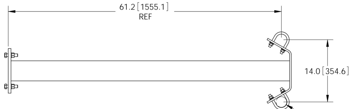
Ø 2.38 O.D. PIPES WITH INCLUDED U-BOLT
