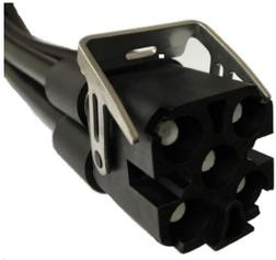
HELIAX® M-LOC Multiport cluster 5 ports SureFlex® cable assembly with interface type M-LOC latching male to 4.3-10 male push pull, size 3/8", length 3 meters
