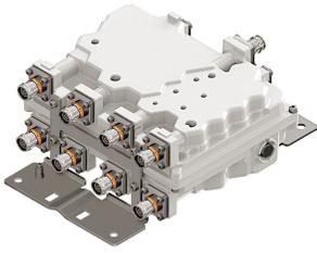
Twin Quadplexer 1800//2100//2300//2600 MHz, All ports DC bypass, with 4.3-10 connectors
