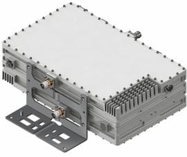
Quad Band TMA 1800/2100/2300/2600, 1 AISG, 4 devices - 2 subunits, with 4.3-10 connectors
