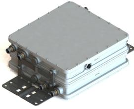
Tri Band Tower Mounted Amplifier, 1800/2100/2600 MHz, 12 dB, 2 BTS & 4 ANT ports, AISG with 1 RET connector (1 device with 2 sub-units each), with 4.3-10 connectors, 698-960 MHz Bypass
