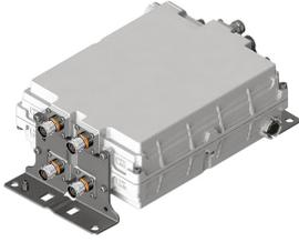
Dual Band Tower Mounted Amplifier, 1800//2600 MHz, 12 dB, 2 BTS & 4 ANT ports, with 4.3-10 connectors, AISG with 1 RET connector (1 device with 2 sub-units each)
