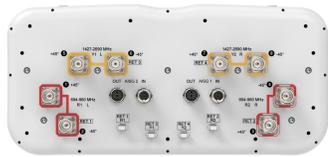
8-port sector antenna, 4 x 694–960 MHz and 4 x 1427–2690 MHz, 65° HPBW, 4x RET
