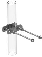
PIM-Guard® Round Member Cable Support Bracket for Block Hangers (pkg of 10)- Two 3/8" threaded rods for up to 12 hangers. Install with torque wrench set at 10 to 15 ft-lb to meet carrier PIM requirements.
