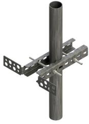
PIM-Guard® Antenna and RRU Cable Support Bracket with 8 ports for stackable hangers (up to 3 per port). Install with torque wrench set at 10 to 15 ft-lb to meet carrier PIM requirements. For patents, see [www.cs-pat.com](http://www.cs-pat.com)
