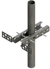
PIM-Guard® Antenna and RRU Cable Support Bracket with 8 ports for stackable hangers (up to 3 per port). Install with torque wrench set at 10 to 15 ft-lb to meet carrier PIM requirements. For patents, see [www.cs-pat.com](http://www.cs-pat.com)
