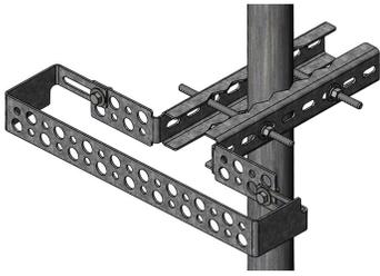
PIM-Guard® Antenna and RRU Cable Support Bracket with 23 ports for stackable hangers (up to 3 per port). Install with torque wrench set at 10 to 15 ft-lb to meet carrier PIM requirements. For patents, see [www.cs-pat.com](http://www.cs-pat.com)
